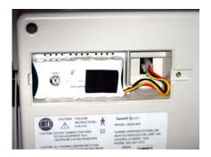
CAUTION: The battery pack contains a temperature measurement component that is matched to the cell type and to the product requirements. Use only replacement battery packs as specified by Summit Doppler Systems, Inc.
