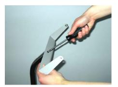
5. Use the two stand mounting knobs to attach the mounting bracket to the Vista **ABI**.
