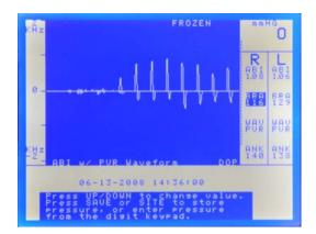
Doppler Waveform During Acquisition of Systolic Pressure
