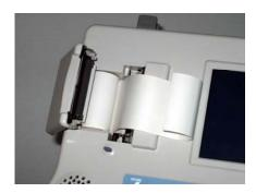
WARNING: Printer components become hot during printing. Do not touch the metal pieces inside the paper holder immediately after printing. After loading paper, press the ON/OFF switch to begin using the instrument.
