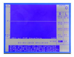
The site will change to DP. Press PUMP to repeat the pressure cycle. Both pressures will be stored and displayed, but the displayed ABI will be either the higher or the lower value depending on the setting.
